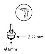
Position the template in the vehicle, remove the center drill and drill carefully down to the honeycomb.
