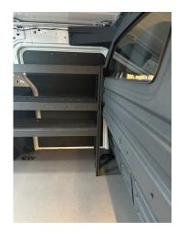
Position the rear bracket (long or short depending on kit) and secure it with two bolts M8x40.
